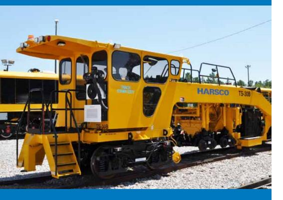
Harsco Rail's Track Stabilizer, Model TS-30, stabilizes the track by inserting controlled and accurate force directly into the track structure. The operator has the ability to set the desired down-feed pressure for each rail and the machine maintains that constant pressure until the operator changes it. The TS-30 Stabilizer reduces slow orders after tie change-out or undercutting operations.
