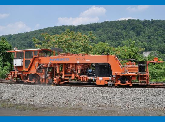
The Mark VI Tamper is designed and manufactured for high-quality production and switch tamping. The machine is equally effective on wood or concrete ties. The Mark VI Tamper is also versatile in configurations of various track gauges. Harsco Rail's tampers are designed to meet customer requirements.
