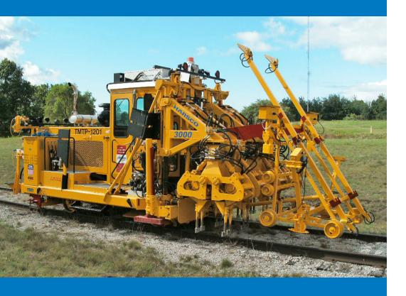
For switches, crossovers or production tamping and lining, the 3000 Utility and Spot Tamper delivers exceptional tamping quality and accuracy. Compact yet powerful, the 3000 is equipped with the same high performance, heavy-duty workheads as our premium 6700 tamper. The benefit to you: outstanding reliability and productivity.
