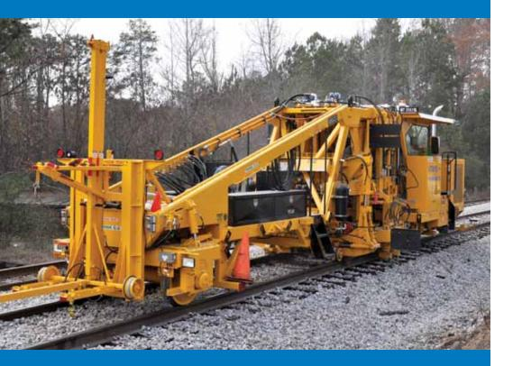
The 6700PD is the latest version of Harsco Rail's well-known production and switch tamper, known for top quality production, switch tamping, and transit system work. The PD model utilizes Harsco's Positive Displacement Workhead Technology and is equally effective on wood or concrete ties. Harsco Rail Tampers are designed to meet customer requirements.
