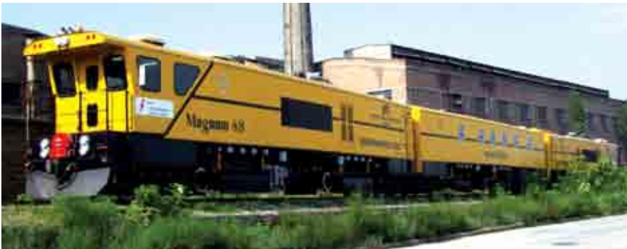
PTG Grinder in the 16-Stone Configuration
