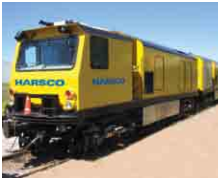
PGM Grinder in the 48-Stone Configuration
