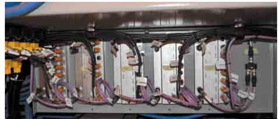
Jupiter II Control System uses remote I/O devices to simplify railway maintenance equipment's electrical control systems
