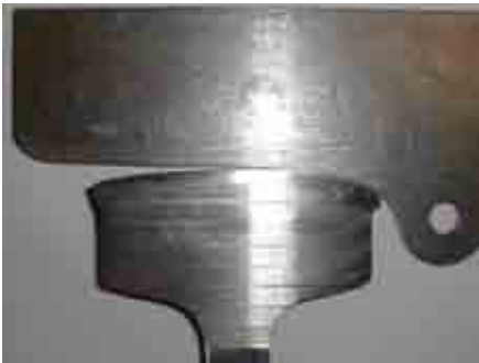
Gauge corner wheel to rail contact before grinding
