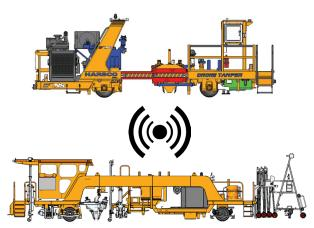
All data transmitted via wireless radios between Lead and Drone
