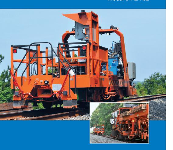
Harsco Rail's Drone Tamper is a 16 tool machine that works with a production / switch tamper and creates a high production, switch capable operation. The Drone Tamper uses Harsco Rail's Jupiter II Control System and Tie Finding System to automatically tamp ties skipped by the lead tamper. A map of the tamped and untamped ties is transmitted via wireless radios from the lead tamper to the Drone.
